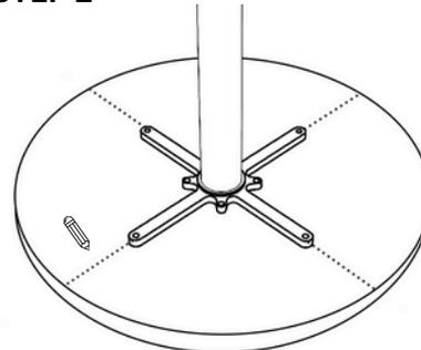
Measure and centre the assembled table base, marking the placement points with a pencil.
