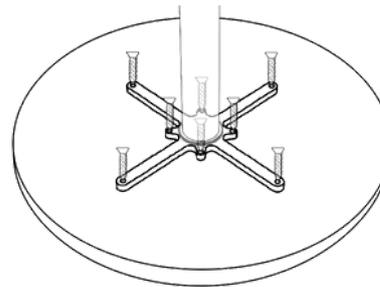
Fasten the screws at the marked positions, ensuring a secure fit. When using a power tool, set it to a low power setting for optimal control.
