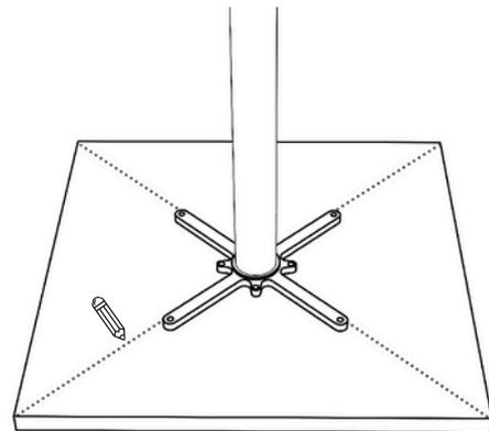
Measure and centre the assembled table base, marking the placement points with a pencil.
