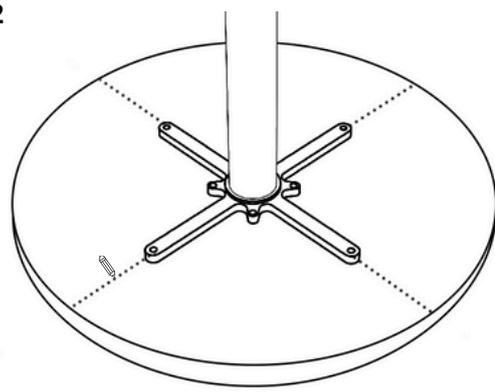
Measure and centre the assembled table base, marking the placement points with a pencil.
