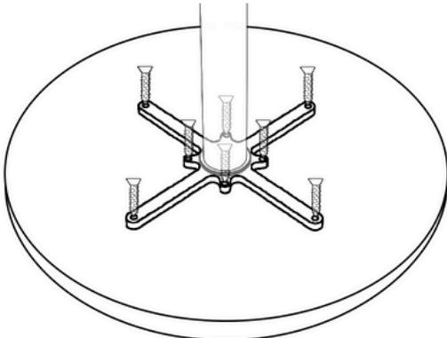
Secure your screws at the marked positions, use the low power setting when operating any power tool.
